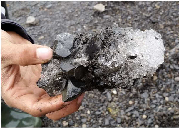
Fig. 13. Rock fall fragment with ice-filled cracks from the active upper rock face of the rock slide, indicating weakening of the rock mass by melting of ice-bonded joints.
